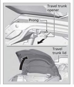
**3.** Install the travel trunk opener onto the prong before closing the right saddlebag.
