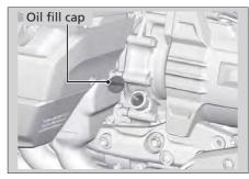
2. Securely reinstall the oil fill cap.
