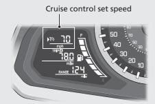
Each quick tap (brief push and release) on either side will change your speed by 1 mph or 1 km/h (depending on mileage meter set unit).
