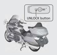
If you press the UNLOCK button, but nobody opens any of the compartments within about 30 seconds or about 30 seconds have passed after an opened compartment is closed, the compartments automatically will relock (Turn signals blinks once).
