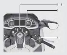
Press the start button with the throttle completely closed.
