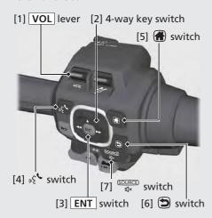
[1] **VOL** (volume control) lever: Push the lever up to increase the volume.
