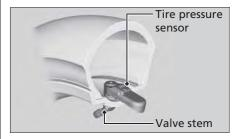
Each tire has its own pressure sensor. If the air pressure of a tire becomes significantly low while riding, the sensor in that tire sends a signal that causes the low tire pressure indicator to turn on.
