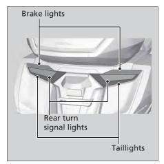
The brake lights, taillights and rear turn signal lights use several LEDs.
