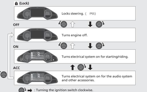
: Turning the ignition switch counterclockwise.
