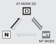
**Neutral (N):** Neutral is selected automatically when you turn the ignition switch to ON.
