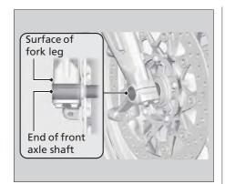
**5.** Install and tighten the axle bolt.
