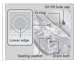
**4.** Install a new sealing washer onto the drain bolt. Tighten the drain bolt.
