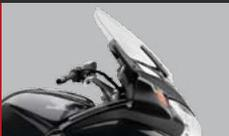
Push-button, electric-motor-driven windscreen can adjust over a wide range of height (7.4 inches) and angle (13 degrees).
